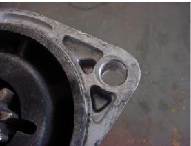
2. Drill out the starter threads using a 13/32" drill bit.
