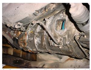
9. Install the supplied driveshaft and the slave cylinder. If you are still using the stock clutch line, you may have to unbolt it from the bracket on the body to give it more slack.
