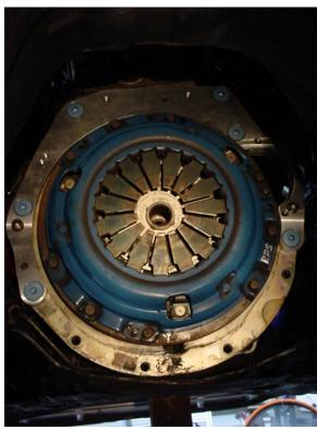
1. After completely removing original KA trans, install the adapter plate and bolts. Make sure that both dowels (one small, one big) are still in the block and that the adapter fits over those dowels to index the plate.
