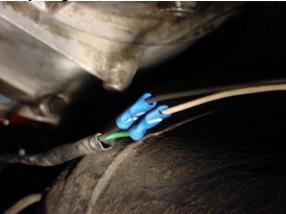
10. To wire up the speedo, cut as muchof wire off of the KA speedo. Plug it into the harness as normal. Cut off the plug on the VG speedo. Wire them together as the picture shows making sure you wire the black wires together. Speed might not read the same.
