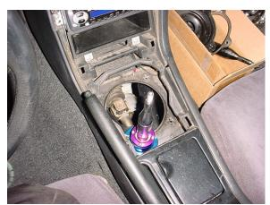
7. Do not install the shifter yet. You will have to locate where the center of the shifter will sit and use a 2" hole saw to trim out the sheet metal. After trimming, you can install the shifter. Make sure you put a little grease on the collar before installing into the bushings.
