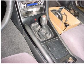
8. Install the cover plate for the tunnel hole. Then replace the interior pieces and screw on the shift knob.
