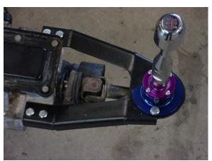
4. Bolt on the Shifter Bracket. Do not install the shifter at this point.
