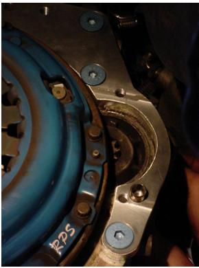
3. Bolt the starter on. The bolts will be threaded into the adapter plate from the engine side.
