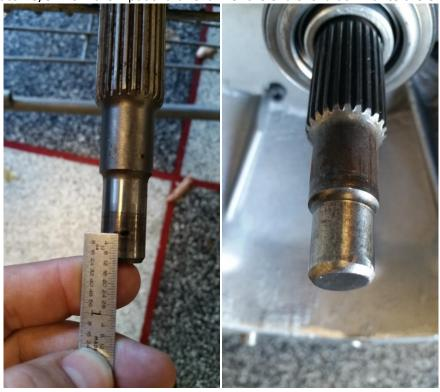
5. Make sure there is no fluid left in the transmission. Remove the stock input shaft front cover and gasket. Clean off are where new gasket will go. If you have an HR or VHR trans, you will need to put the adapter ring (sold separately) over the large bearing before installing the bell housing. Use new gasket and install bell housing. Torque bell housing bolts to 13 ft-lbs.
